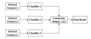
Fig.1. Block Diagram of Multi-classifier System [17]
